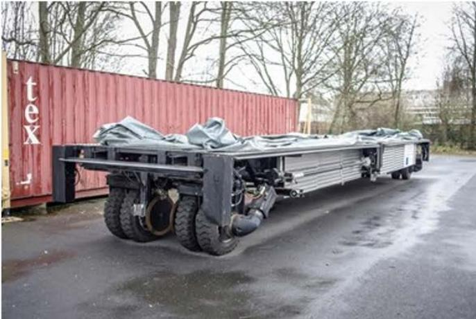
(a) Robutainer autonomous redundant vehicle
